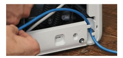
• Connect the ethernet cable to the RJ-45 receptacle (network input connector or port) in the kiosk as shown here:
