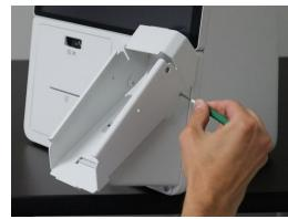
Next remove the two screws from the underside of the right side of the mount as shown here:
